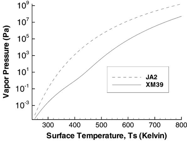
Fig. 1. Calculated vapor pressure for each propellant.
