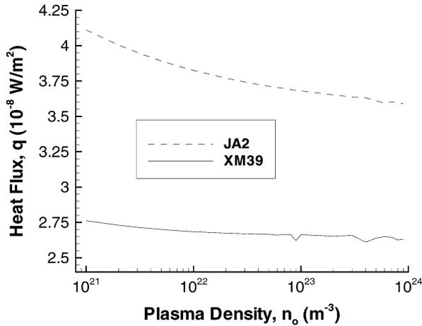
Fig. 6. Effective plasma heat flux to each propellant predicted by model, where the ablated mass equals the experimental value.
