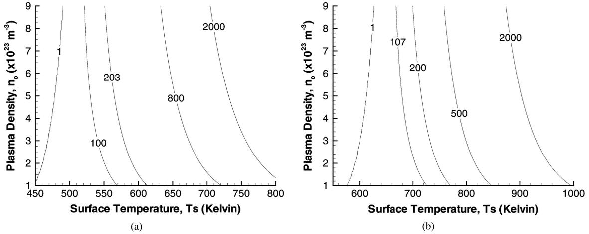
Fig. 5. Ablation rate contours for each propellant. (a) JA2. (b) XM39.
