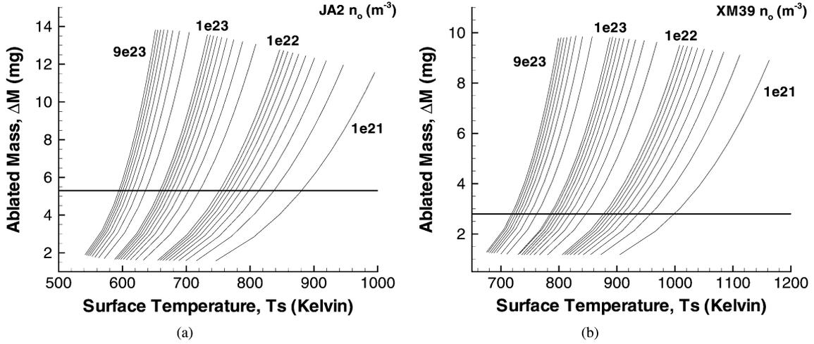
Fig. 4. Simulation results for ablated mass versus propellant surface temperature. (a) JA2. (b) XM39.
