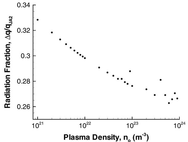
Fig. 7.  $\Delta q/q_{\text{JA2}}$  the dependence of the fraction of radiation flux on the plasma density in the vicinity of the propellant.
