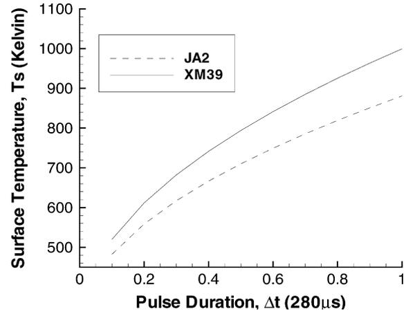
Fig. 2. Representative surface temperature versus increments of plasma pulse duration for each propellant that matches their respective experimental ablated masses at  $n_o = 1 \times 10^{21} m^{-3}$ . Effective heat fluxes are  $4.1 \times 10^8 W/m^2$  and  $2.75 \times 10^8 W/m^2$  for JA2 and XM39, respectively.
